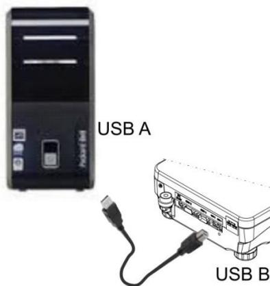
3. The system detects the new USB device and automatically starts searching for a respective driver.
