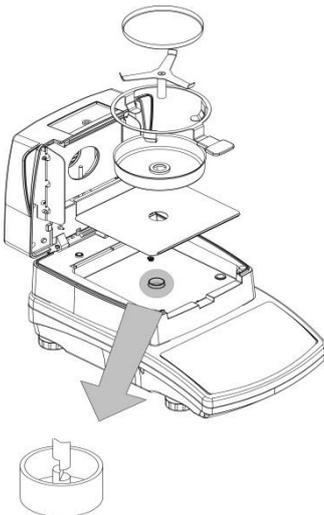
When installing the cross-shaped holder (pan supporter) pay special attention to the correct positioning of its mandrel. The mandrel features a cut providing unique positioning of the holder against the pan handle, thus preventing their contact and friction.
