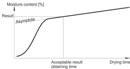
The sample undergoes thermal decomposition, wherein evaporation takes place and as a result the product weight decreases. Evaporation of grease, oil, plastic or other volatile materials may take much more time than in case of water. Difficult to evaporate materials drop weight.
