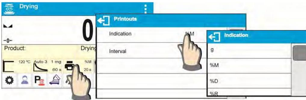
**g** - mass change; measurement result is mass change recorded during drying process.
