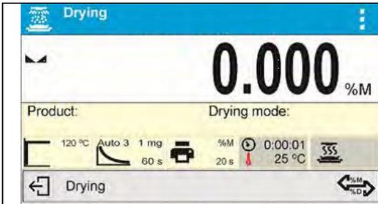
Information on the drying process is displayed, moisture analyzer proceeds to carrying it out accordingly to set parameters. Required mass measurements and calculations of tested sample moisture content are performed, wherein the calculations are a result of mass change. Upon process start, printout header is sent to a selected interface (accordingly to set printout options – parameter group DRYING PROCESS REPORT/HEADER).
