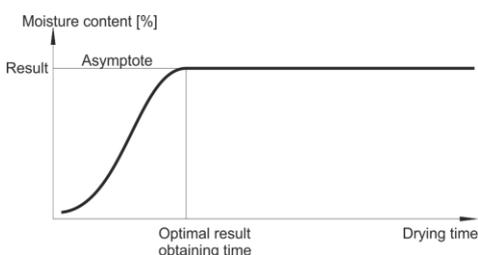
For the second case the drying process is quick at the beginning, next it stabilizes. Moisture content value is never constant. The properties of the sample may cause it.
