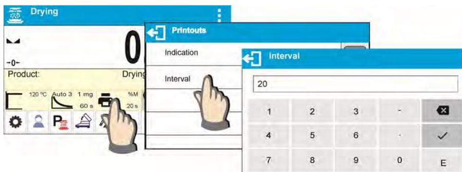
The time interval between printouts in seconds ranging from 0 to 120.
