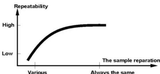
Final measurement result is vastly conditioned by precise and considered sample preparation. A sample used for analysis has to represent the total structure of tested material. Sampling process should determine: sampling means, sample disintegrating, particle size after disintegration, sample uniformity and other. The sampling process has to be carried out as quickly as possible, so that a sample does not lose or absorb moisture from surrounding area.
