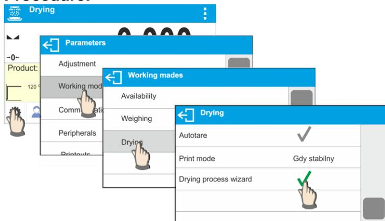
Enable the function to activate drying process wizard. The wizard guides you through all steps of setting the drying parameters. Only after setting confirmation the moisture analyzer will start the process of sample preparation and drying.
