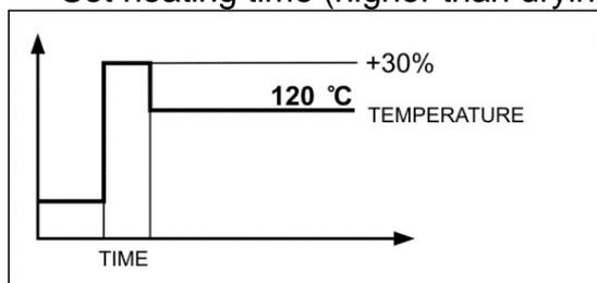
Specific feature of this drying profile is fast increase of drying temperature in short period of time. When compared to the preset temperature, the drying temperature rises 30% within 180 seconds and it is maintained at this level for a specified amount of time, next it drops to temperature value preset in drying profile parameters.
