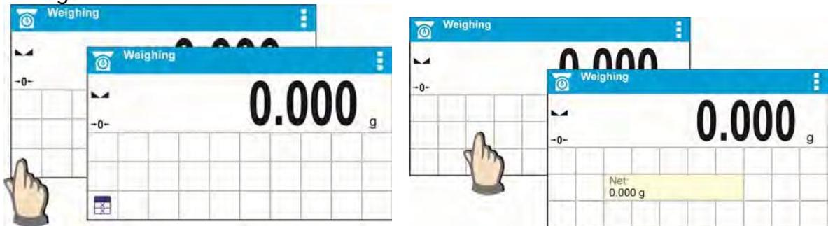
3. A new widget can only take such area that holds no other widgets yet. The program automatically detects suitable widget size matching particular area.
