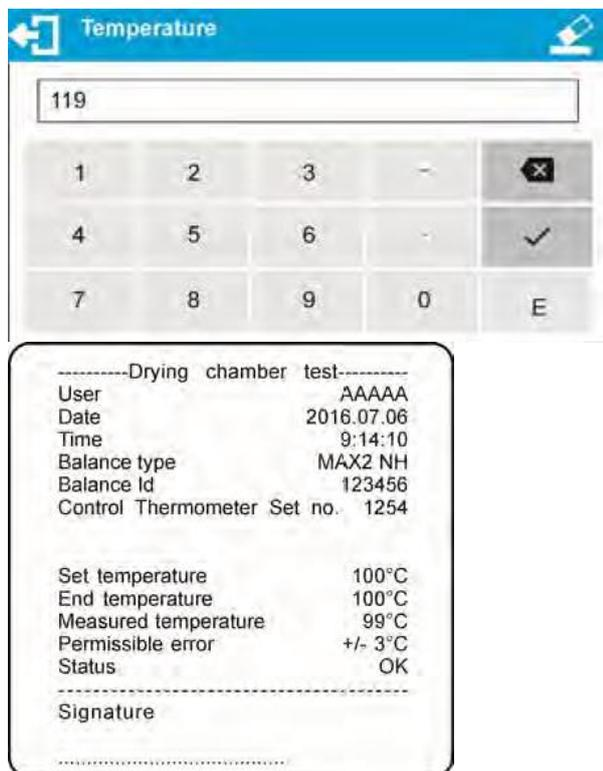
The temperature is maintained for 8 minutes (like for temperature adjustment procedure). After 8 minutes you shall see a window for entering temperature read from the installed adjustment set. Press ✓ button to confirm.
