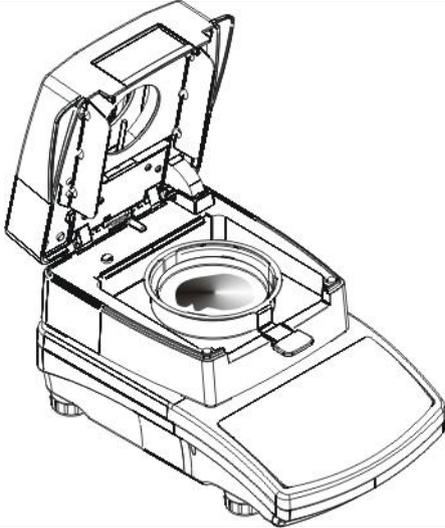
Load the weighing pan with the sample. Sample mass shall be selected on the basis of prior experience and tested material characteristics.
