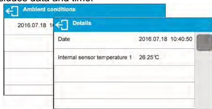
*Caution: The software saves ambient conditions record in a so called loop, i.e. when the measurement 10 001 is saved, the measurement 1 gets automatically deleted from the moisture analyzer memory.*
