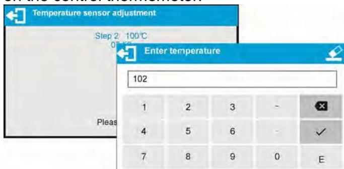
Press ✓ button to confirm, the third step of adjustment starts. The moisture analyzer halogen lamp starts to operate and the drying chamber is heated as long as necessary to provide specified temperature, which is next maintained for 8 minutes. After 8 minutes a
