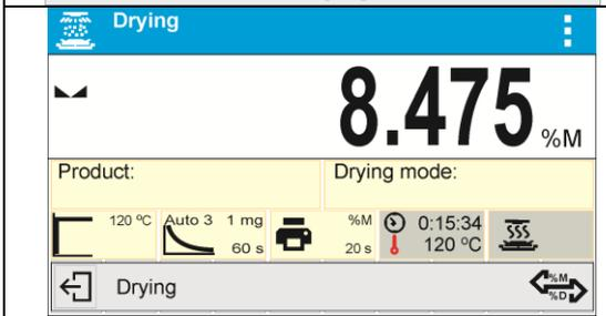
In course of a drying process current weight results and information on the process is displayed (test duration, drying chamber temperature, etc.). In course of a drying process (accordingly to set printout options – parameter group DRYING PROCESS REPORT/MEASUREMENT) measurements are sent to a selected communication port in a preset time intervals (INTERVAL).
