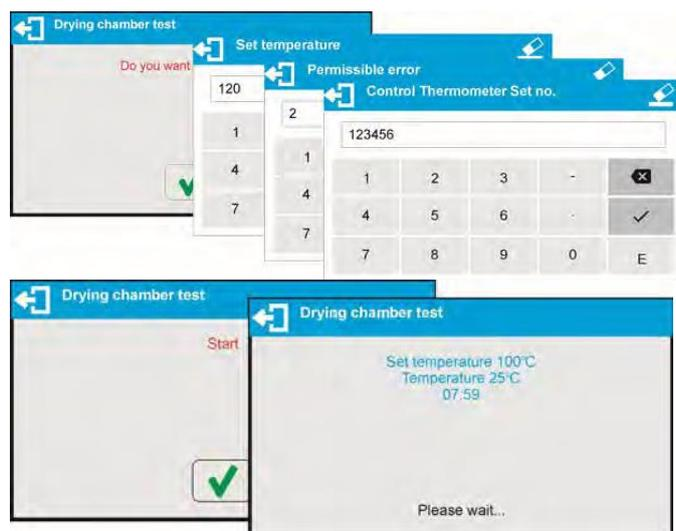
Enter testing temperature, maximum permissible error and the serial number of the temperature adjustment set.
