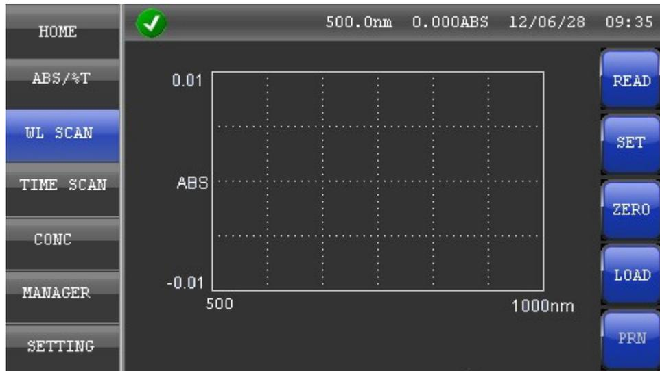
Wavelength scan allow scanning the sample transmission, absorbance and energy (for service purpose).
