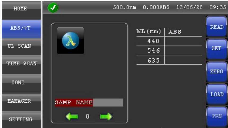
Photometry function can measure up to 6 selected wavelength's absorbance or transmission. Each measurement file can store up to 200 results.
