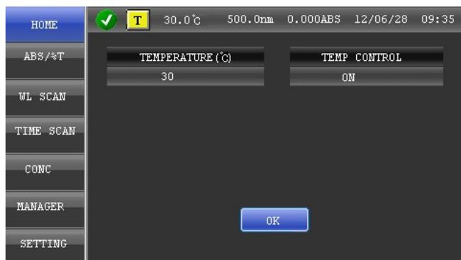
TEMPERATURE (°C):      Setting control temperature
