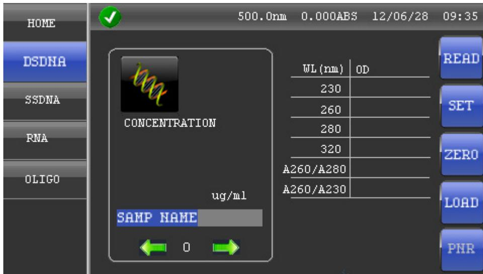
There are 4 methods in the DNA/RNA nucleic acids analysis interface, dsDNA, ssDNA, RNA, OLIGO. Click button to select measure method.
