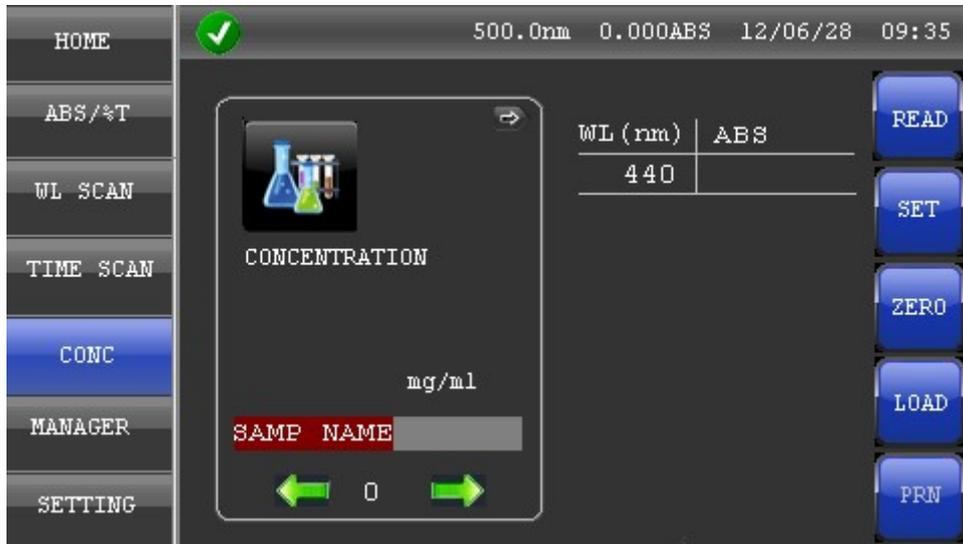
Concentration or specified wavelength can be measured. Up to 5 wavelengths can be chosen. Up to 9 standard and 5 replicates can be recorded. Standard curve and its K-factor value are displayed. The standard curve data can be input for known concentration curve. Standard curve can be saved in the SD card. Each file can store up to 200 results.
