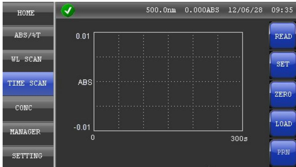
Time scan can scan the sample transmission, absorbance with a specific wavelength and within set time.
