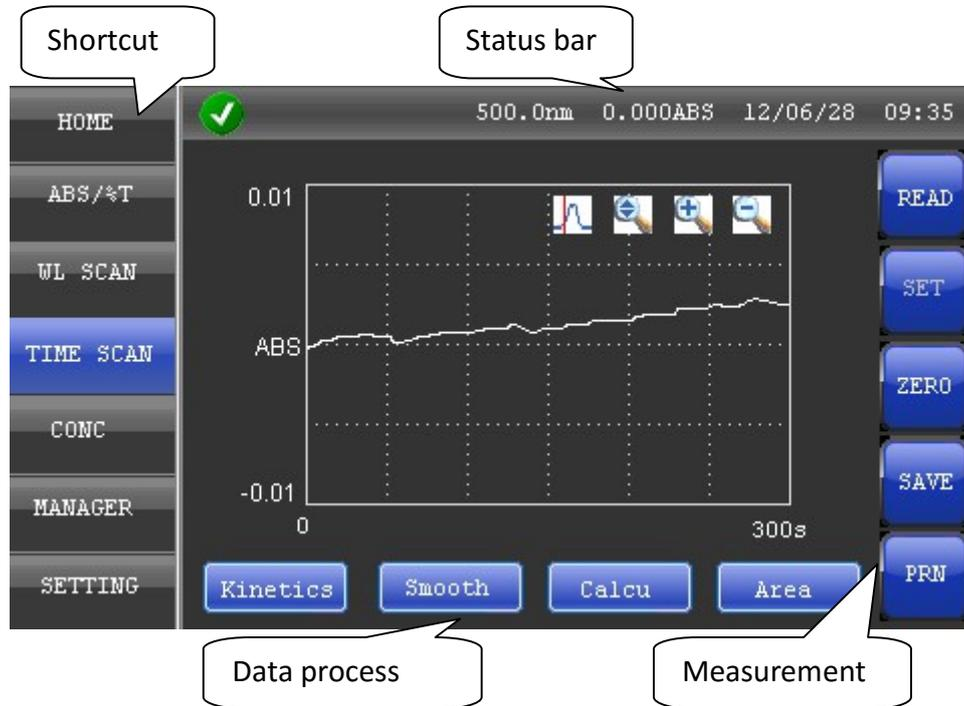
**Shortcut** appear on every interface and can quickly switch to different measurement functions.
