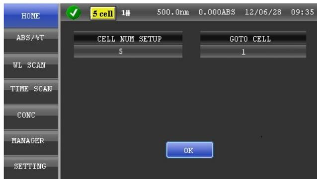
CELL NUM SETUP: Cuvette position to be measured (1 to 5 )
