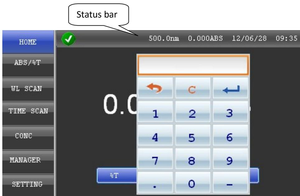
Click wavelength in the status bar, input wavelength, the instrument will go to the select wavelength for measurement. (GOTO  $\lambda$  function)
