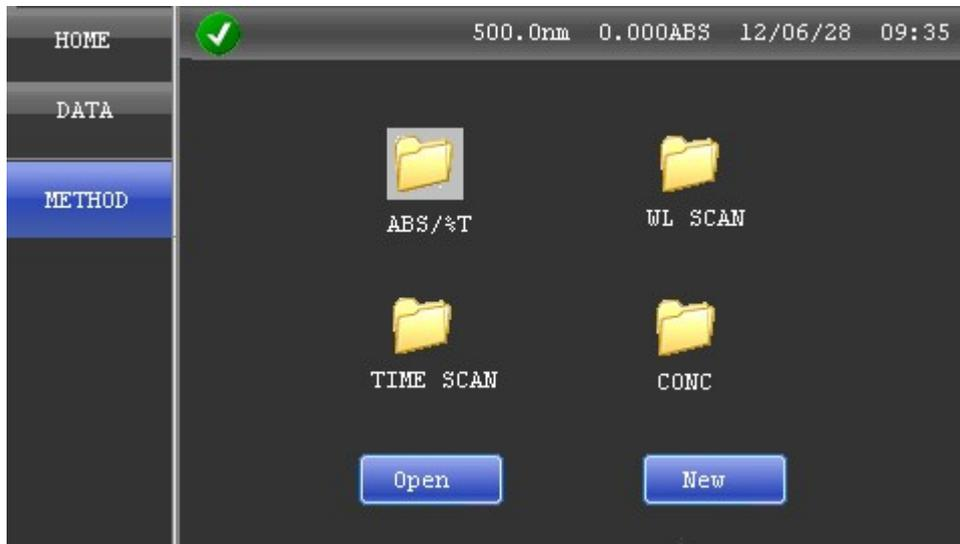
Method Manager is designed for managing all method files. SD card must be inserted for storing and opening the files.
