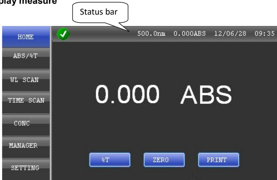
The large display can be used to measure single wavelength's absorbance or transmission. Click the value in the status bar in any screen can enter the large character measure mode.
