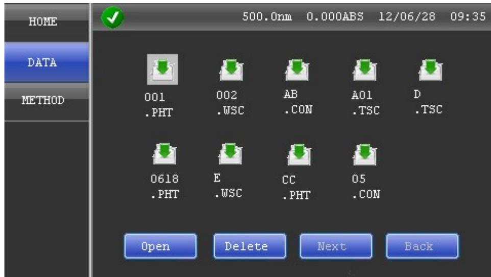
Data manager function is designed for managing all data files. SD card must be inserted for storing and opening the files.
