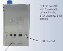
input for alkaline detergent for automatic cleaning on every hour
