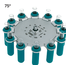
Swing-out rotor, 12-place, n= 5,000 min -1 , max. RCF 4,193, for 12 x 15 ml, stainless steel, with suspensions No. 01621, PA, fibreglass reinforced.
