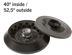
Angle rotor, 30-place, Cat. No. 02437 n = 15,000 \text{ min}^{-1} , max RCF 21,328 incl. bioseal lid.
