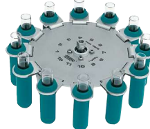
Swing-out rotor, 12-place, n = 5,000 min -1 , max. RCF 4,193, for 12 x 15 ml, stainless steel, with suspensions No. 01621, PA, fibreglass reinforced.
