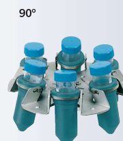
Swing-out rotor, 6-place, n= 4,000 min -1 , RCF 2,701, for 6 x 50/15ml Falcon tubes, stainless steel, with suspensions, PA, fiberglass reinforced.
