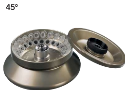
Angle rotor, 24-place Cat. No. 02428 n = 15,000 \text{ min}^{-1} , max RCF 21,382 incl. bioseal lid
