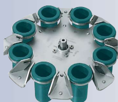
Swing-out rotor, 8-place, n = 4,000 min -1 , max. RCF 2,415, for 8 x 15 ml, stainless steel, with suspensions No. 01644, PA, fibreglass reinforced.
