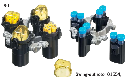
Swing-out rotor, 01554, 4-place, illustrated with carrier 01560 and lids 01561 n = 4,500 \text{ min}^{-1} , max. RCF 3,328 for max. 4 x 200 ml
