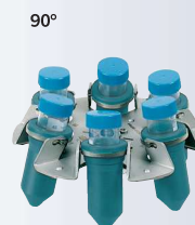
Swing-out rotor, 6-place, n = 4,000 \text{ min}^{-1} , RCF 2,701, for 6 x 50/15ml Falcon tubes, stainless steel, with suspensions, PA, fiberglass reinforced.
