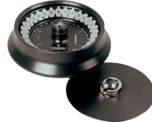
Angle rotor, Cat. No. 01553 30-place, incl. bioseal lid, phenol resistant n = 14,150 \text{ min}^{-1} max RCF 21,713
